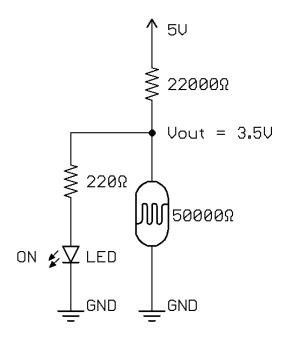
• What should we do with the top resistance in the divider if the LED is still on when the room is bright? Should we make it bigger or smaller to lower Vout so the LED is off? A: increase the resistance of the top resistor.
